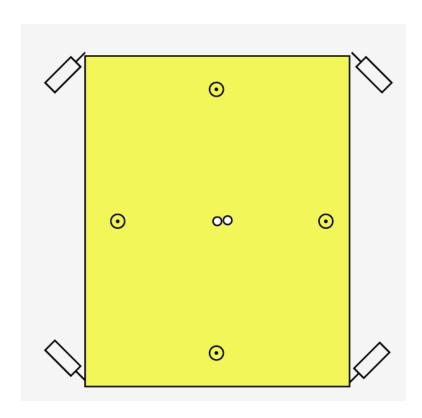
Positioning of sensor-actuators on the intermediate mass. Four vertical actuators are used for vertical, tip and roll modes. Four tangential sensor-actuator are used for yaw, longitudinal and transversal motion control
