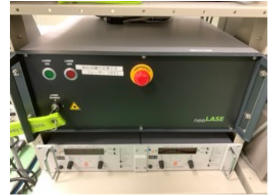
Laser controller ( upper ) and power supply ( lower )
