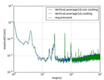
The fluctuation of magnetic field didn't change so much while the cryocoolers were moving.
