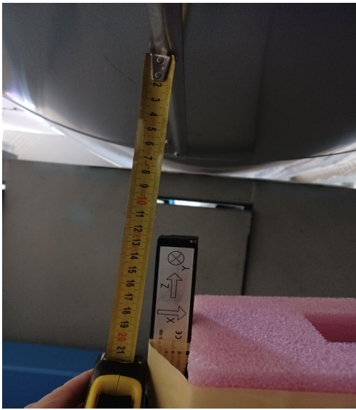
Z along the vertical direction At 13cm distance from the Al tube
