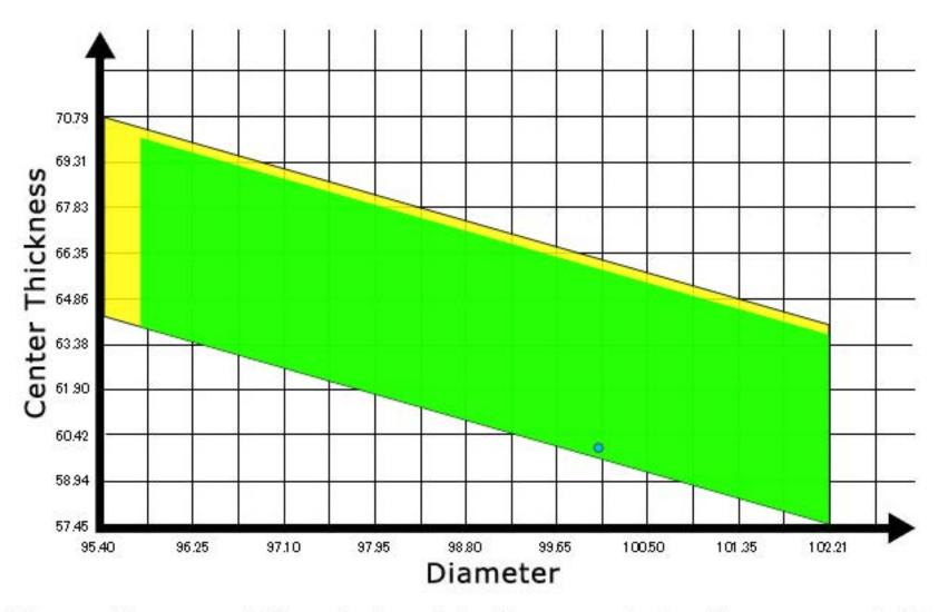
This container provides an acceptable packaging solution for any round, plano/plano component with thickness and diameter dimensions that fall within the shaded area.
