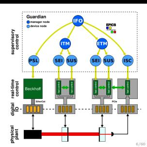
A hierarchy of nodes control the full interferometer.
