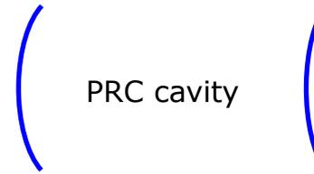
$$\begin{aligned} L_{34} &= 73.3 \text{ m} \\ R_1 &= -1906.2258 \\ R_2 &= 1960.7954 \end{aligned}$$
