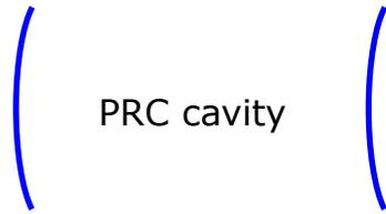
$$\begin{aligned} L_{34} &= 73.3 \text{ m} \\ R_1 &= -7113.9 \\ R_2 &= 6926.359 \end{aligned}$$
