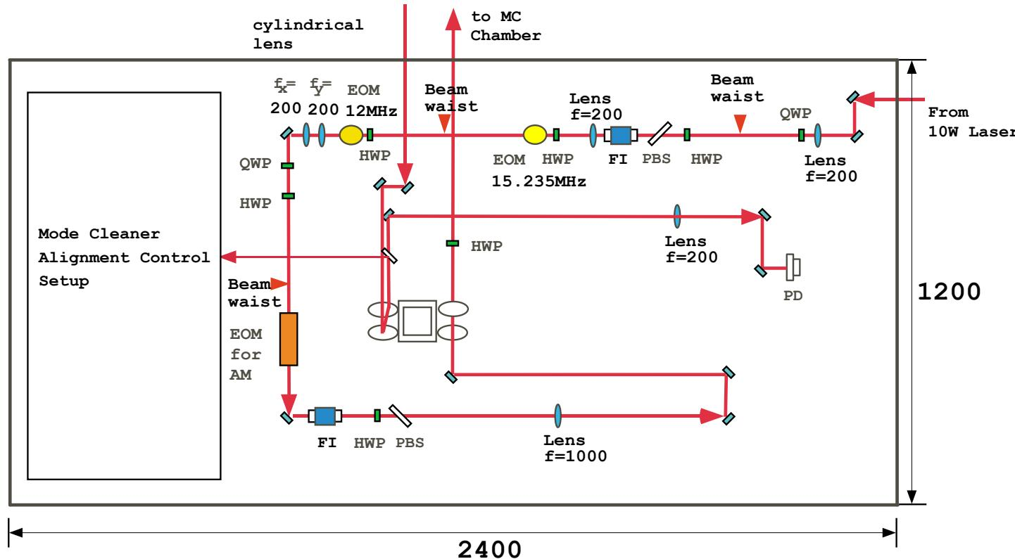
Figure 6.7: Optical configuration on the injection bench to the mode cleaner:
