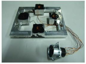
Problem: Eddy current in aluminum coil holders induced by magnets attached on mirror added mechanical loss on pendulum thermal noise
