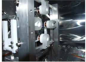
Solution: Aluminum holders were exchanged to ceramic and daifron holders.
